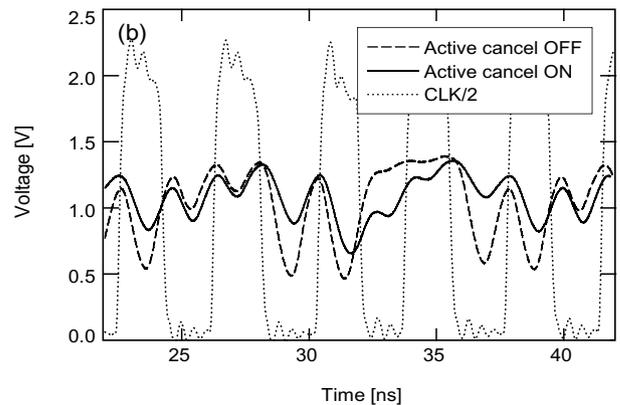
Fig. 7. Substrate noise waveforms with the active noise cancelling ON/OFF, together with the  $CLK/2$  signal. The operating frequency is 500MHz. (a) Repeat mode, and (b) Random mode.
