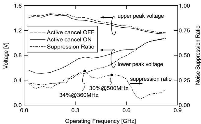
Fig. 8. The frequency dependence of the upper and lower peaks of the substrate noise voltage, together with its suppression ratio by the feedforward active noise cancelling, on the repeat mode.
