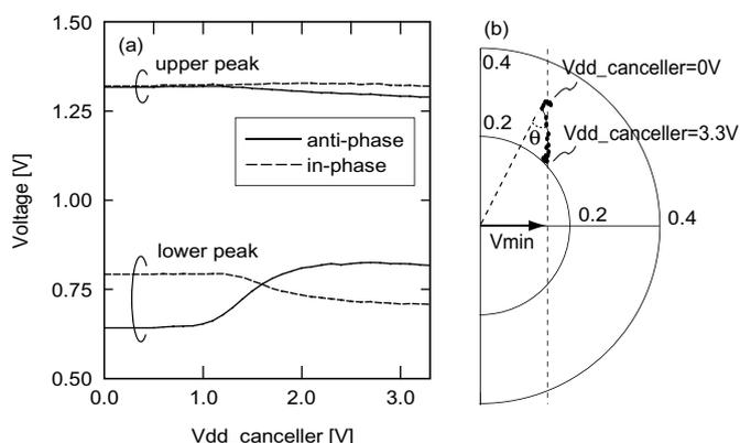
Fig. 9. (a) Noise canceller supply voltage dependence of the substrate noise amplitude, and (b) Phasor of the substrate noise, sweeping  $V_{dd\_canceller}=0V$  to 3.3V by 0.1V step, on the repeat mode at 500MHz operation.
