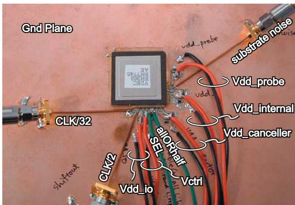
Fig. 6. Photograph of the chip mount.
