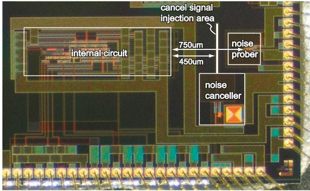
Fig. 5. Chip photograph of the feedforward active noise cancelling circuit, using 0.35 $\mu\text{m}$  CMOS process. The area is 3.0mm $\times$ 1.8mm.
