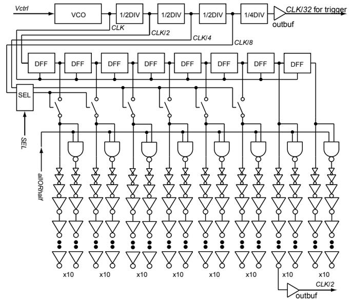
Fig. 4. Internal circuit as a noise source.
