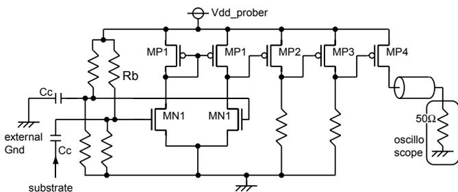
Fig. 3. Substrate noise prober.
