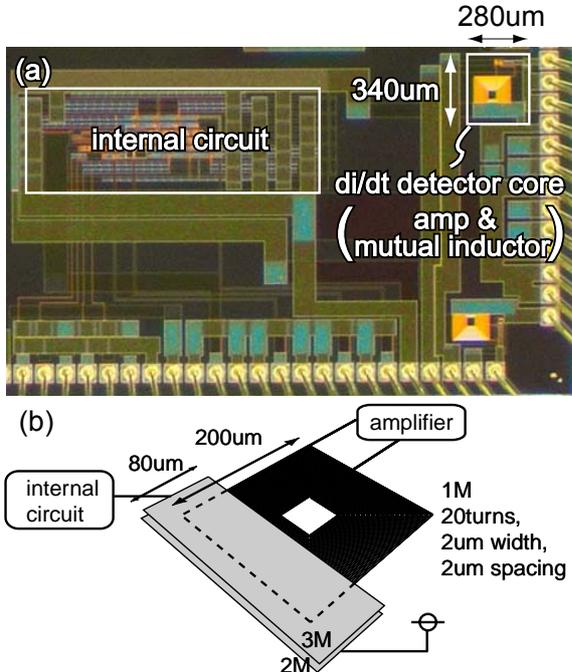
Figure 3: (a) Chip photograph. The chip area is  $3.0\text{mm}\times 1.8\text{mm}$ . The area of the  $di/dt$  detector core is  $340\mu\text{m}\times 280\mu\text{m}$ . (b) Mutual inductor structure.
