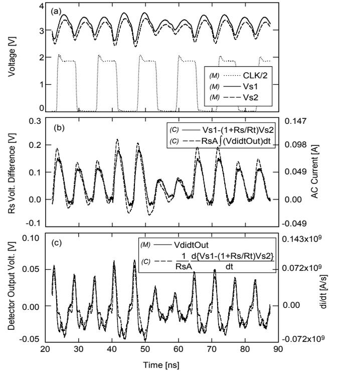
Figure 4: Waveforms of (a)  $CLK/2$ ,  $s_1$  and  $s_2$ , (b) Current waveforms, (c)  $di/dt$  waveforms.
