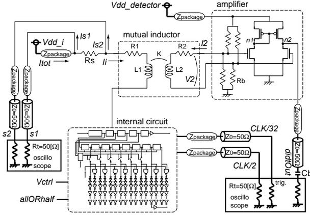
Figure 2: Over-all circuit with the measurement setup.
