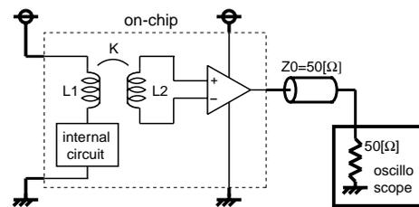
Figure 1: Block diagram of the  $di/dt$  detector circuit. The bold lines represent outside devices.
