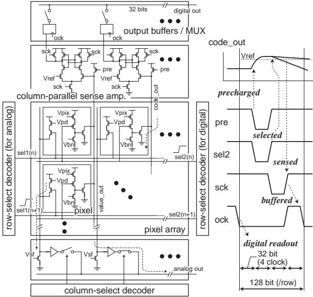
Figure 5. Analog/Digital Readout Circuit and Operation
