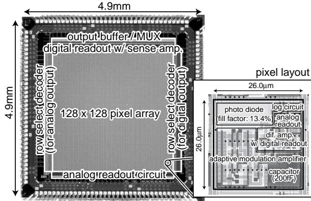
Figure 6. Chip Microphotograph and Pixel Layout
