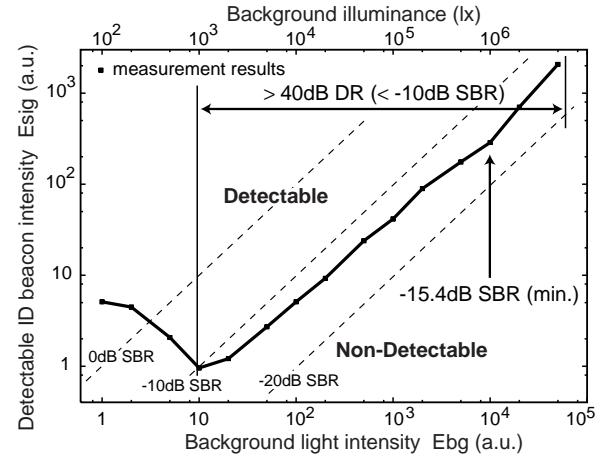
Figure 10. Sensitivity and Dynamic Range of ID-Beacon Detection
