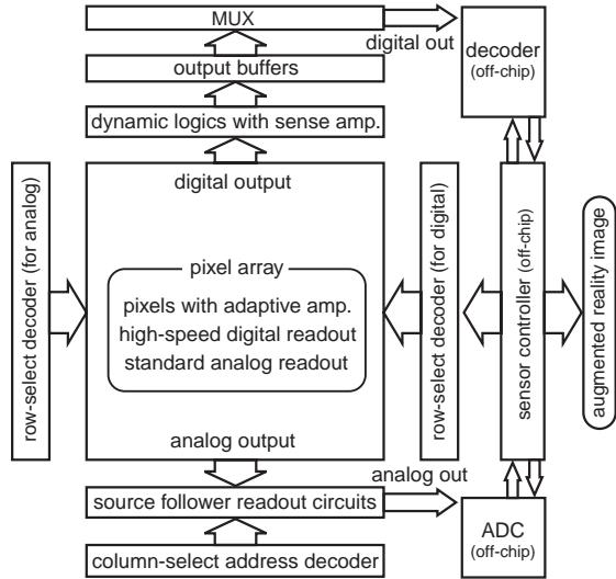
Figure 2. Block Diagram of the Smart Sensor
