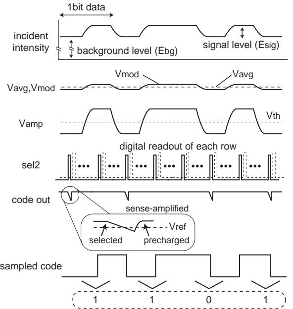
Figure 4. Timing Diagram of the Pixel
