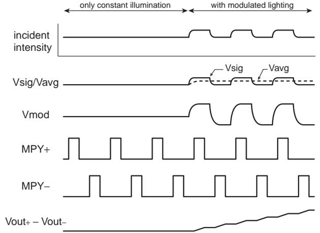
Figure 3. Timing diagram of the sensing scheme.
