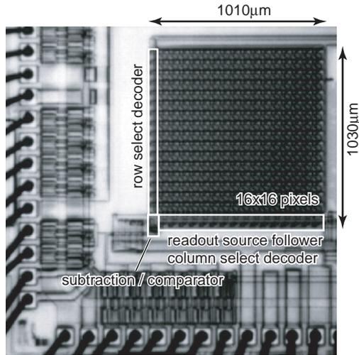
Figure 4. Microphotograph of the fabricated chip.
