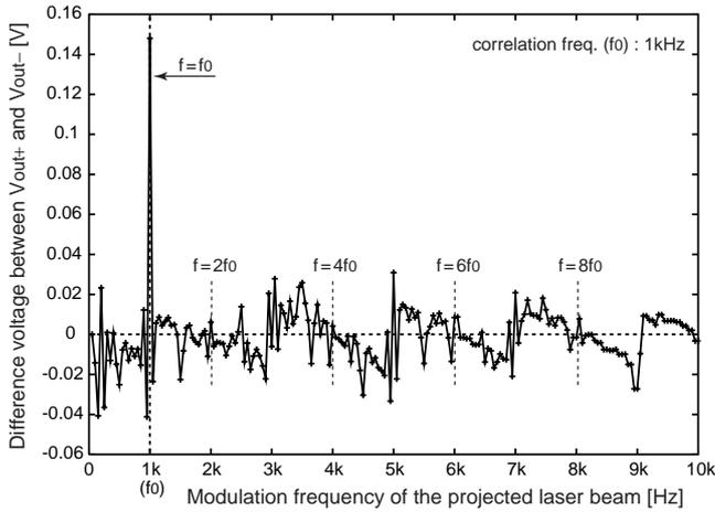
Figure 12: Difference voltage of the correlation outputs at various input signal frequencies.
