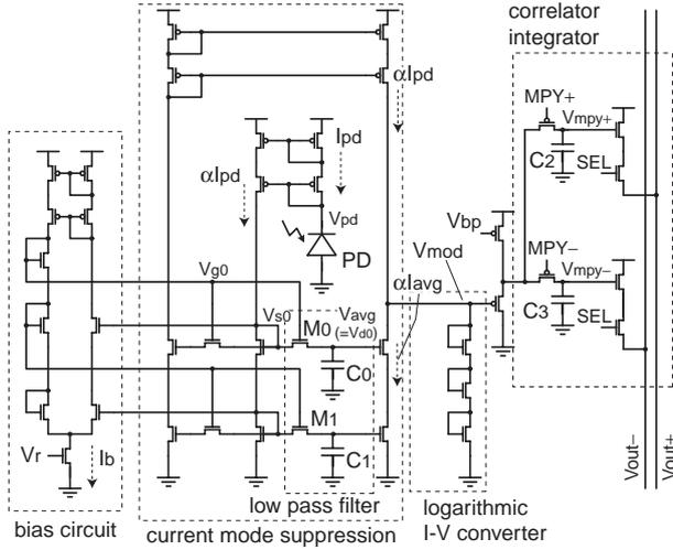
Figure 2. Schematic of the photo detector.
