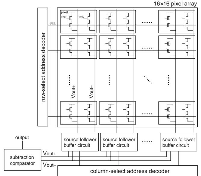
Figure 6. Array structure of the position sensor.
