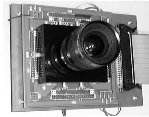
**Figure 10. Photograph of the sensor on a test board.**
