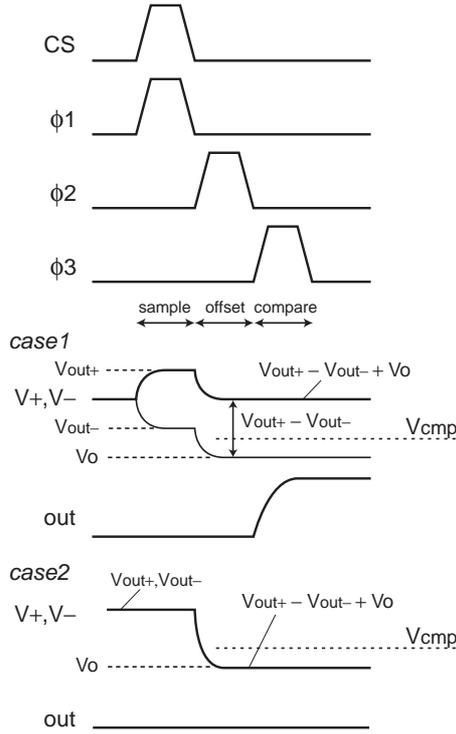
**Figure 8: Timing diagram of the subtraction and comparator circuit.**
