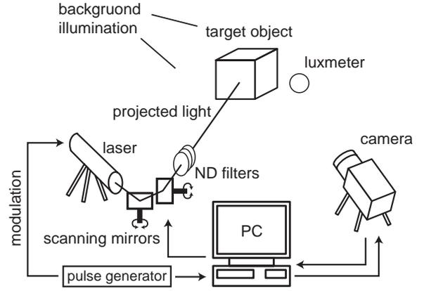
**Figure 9. Measurement system structure.**
