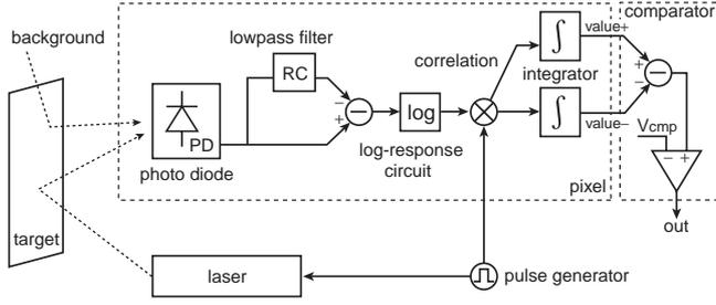
Figure 1. Proposed sensing scheme.
