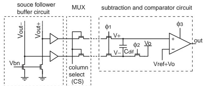
Figure 7: Schematic of the subtraction and comparator circuit.
